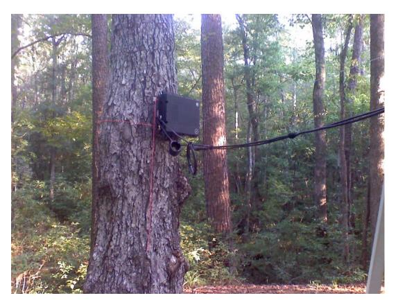
This is the camping setup. Notice the chokes feeding the coupler. I have a SO-239 barrel connector right after the 5" choke for my feed line to the radio.
