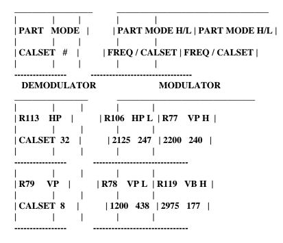
**NOTE!** Separate procedure required to do alignment of CW demodulator center frequency.
