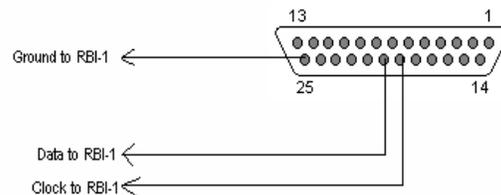
Using the Kenwood TM-V7 or TM-G707 as your remote base radio, a separate hardware interface is required.
